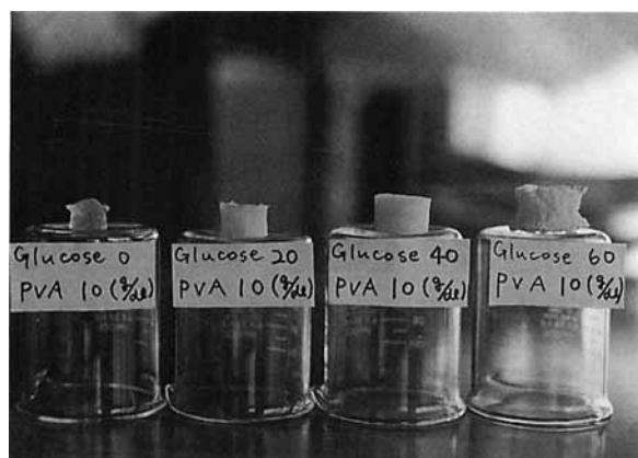
Figure 7 Photograph of gels with or without saccharose after standing for 50 days in air (initial polymer concentration: 10 g/dL).
